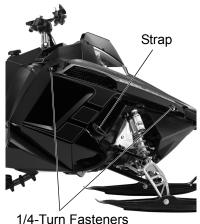
Removing the hood is not recommended. Any service requiring the removal of the hood should be performed by an authorized Polaris dealer
